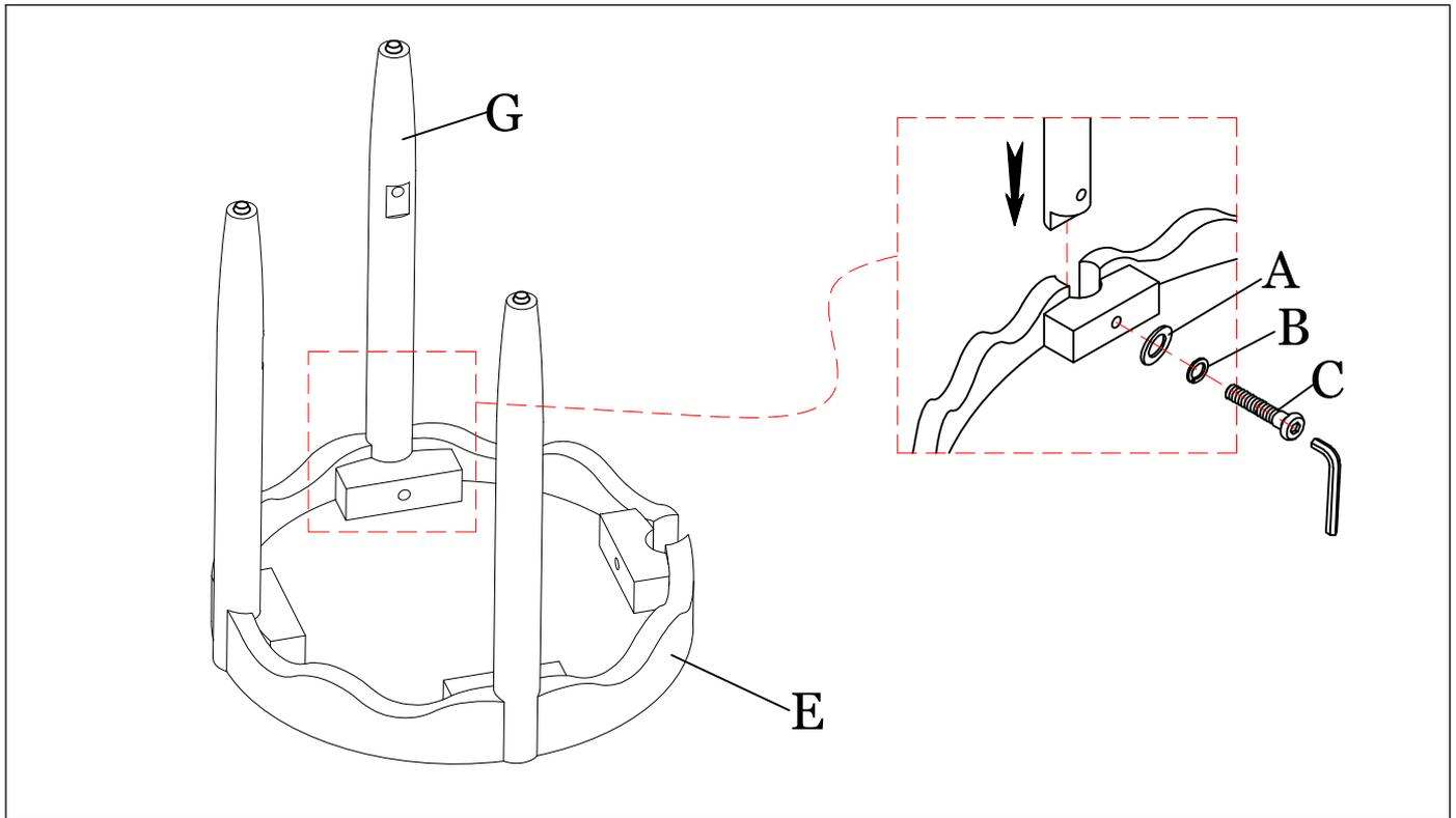
STEP 2: Attach bottom Shelf (F) and Leg (G) on the Table of Step 1 by using Flat washer (A), Lock washer (B), Bolt (D) with Allen key.
