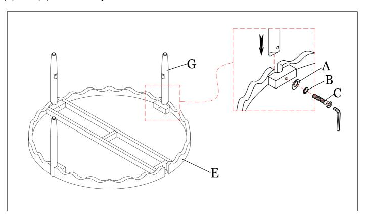
STEP 2: Attach bottom Shelf (F) and Leg (G) on the Table of Step 1 by using Flat washer (A), Lock washer (B), Bolt (D) with Allen key.
