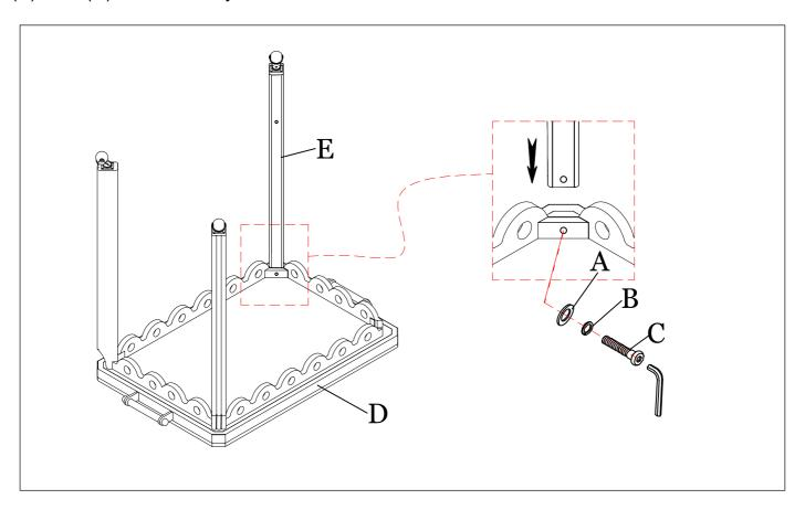
STEP 2: Attach bottom Shelf (F) and Leg (E) on the Table of Step 1 by using Flat washer (A), Lock washer (B), Bolt (C) with Allen key.
